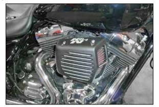
13. Install air filter and air filter cover with provided bolts.
