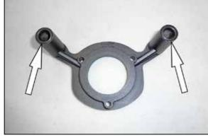
8. Install two o rings provided onto the back side of the K&N $^{\odot}$  back plate as shown.
