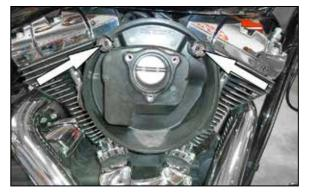
2. Remove the air filter cover retaining bolt and then remove air filter cover as shown. Some models may have a number plate covering the bolts, if so firmly grip edge and remove.
