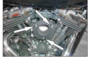
11. Install the provided gasket between the throttle body and back plate use the provided hardware to secure the back plate to the throttle housing. Tighten the crankcase breather bolts. **NOTE: Apply one drop of the provided thread locker onto the provided bolts.**
